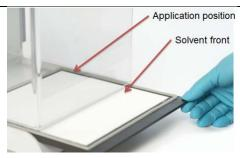
Insert the plate with the solvent front facing the front of the instrument.
