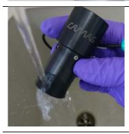
When necessary or when changing the reagent rinse the tip of the nozzle and the inside of the reagent container with (tap) water, ethanol or cleaning solution.
