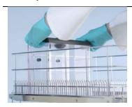
The hood and the tray can be cleaned manually (e.g. with ethanol 96 %).
