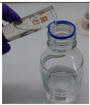
Dilute 10 mL of the aqueous NaCl solution in 90 ml ethanol.
