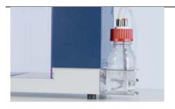
In the reagent evacuation phase, fumes are withdrawn from the hood with the internal pump and absorbed in the washing bottle. This step lasts for one minute but can be shortened by pressing the "START" button.
