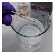
Dissolve half of a spatula (~ 300 mg) of sodium chloride (NaCl) in 500 mL water.
