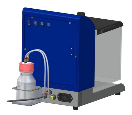
• If the instrument is not placed in a fume hood, connect the output air pipe (grey rear connector) to the fume hood
