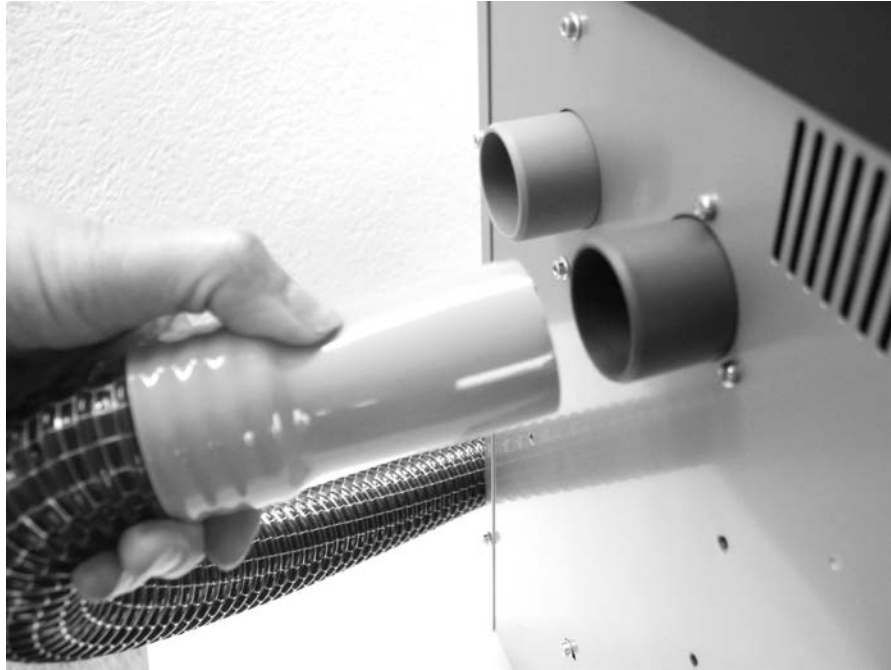
Fig. 4: Mounting the exhaust tube to the air outlet
