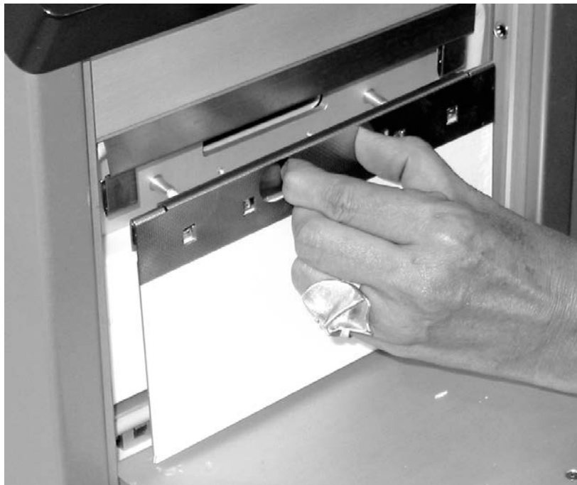
Fig. 8: Fixation of plate holder in drying module
