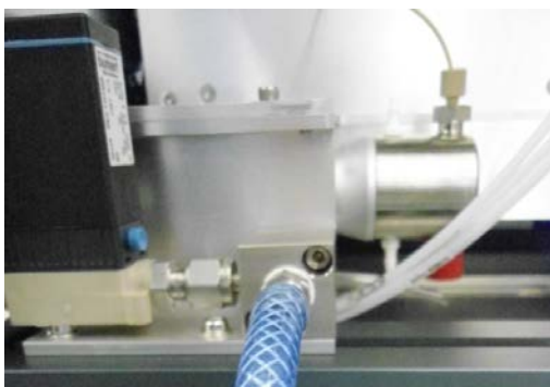
Fig. 1: Waste canister connection
